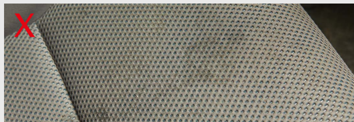
Staining to seat
