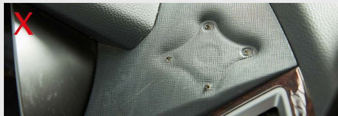
Holes in trim
